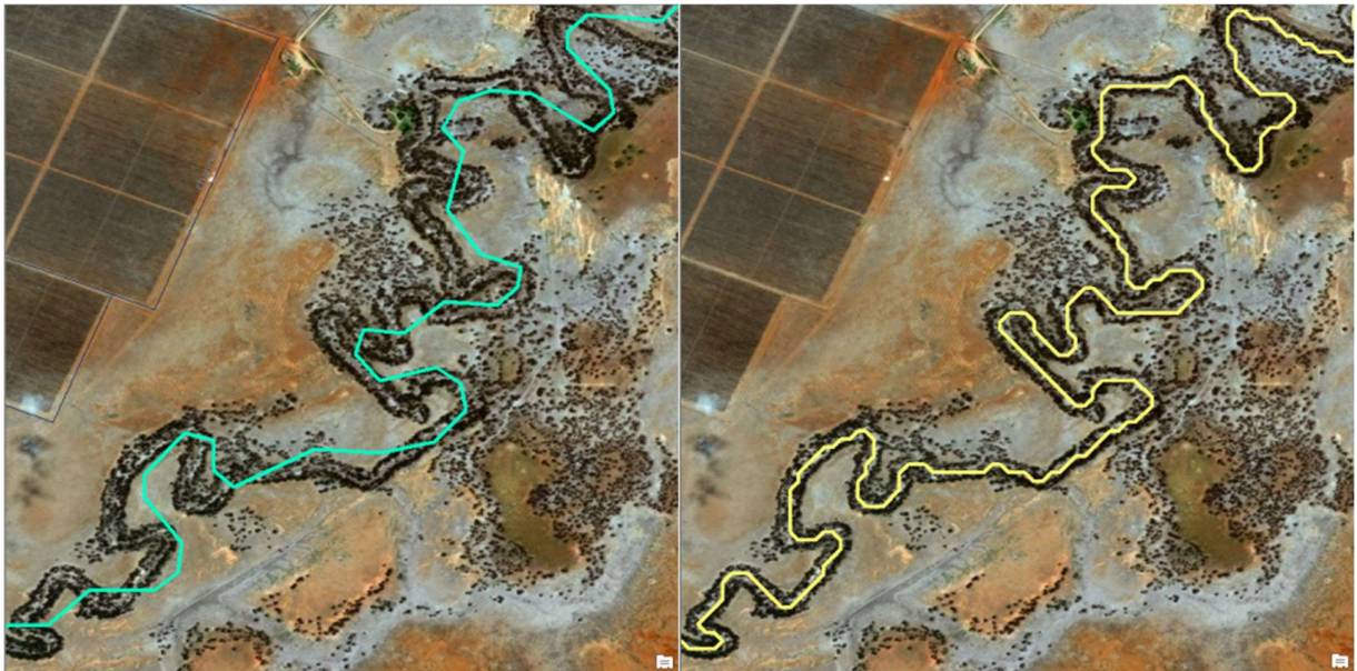
Figure 8: ANAE_Geofabric v2 mapped streams (green) compared to the new higher resolution Geofabric v3 (yellow). The new mapping improves alignment with riparian ecosystems.
