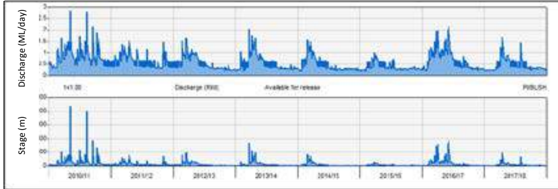
Figure 1. Stream water levels (m) and discharge (ML/day) on the King River at Cheshunt from T1 (03 rd May 2010) until T3 (08 th April 2018).
